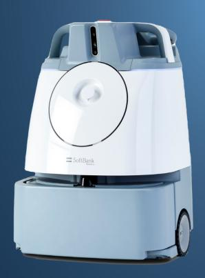
Whiz is an autonomous cobotic vacuum cleaner that collaborates with cleaning teams to create happier, healthier environments. Whiz handles vacuuming and efficiently removes dust, making your spaces safer and giving your staff more time for essential cleaning tasks.
