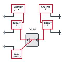
Two FAST BBD models are available offering 2800A and 4800A inrush current ratings which are suitable for a wide range of loads such as Engine Cranking, Switchgear Tripping and Communications and suitable for Voltages from 12 to 150VDC nominal.
